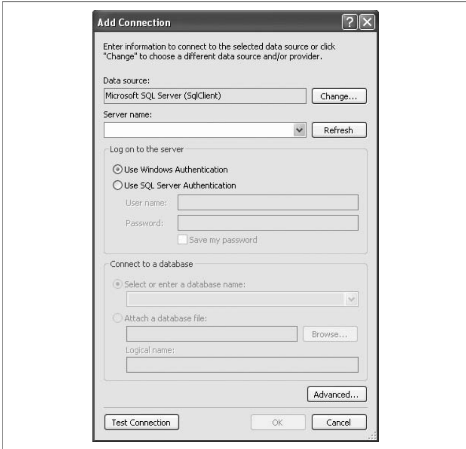
Figure A-5. VWD Add Connection dialog box. Enter the name of the SQL Server instance as the Server name, select Windows Authentication, and select the database name to connect to.
